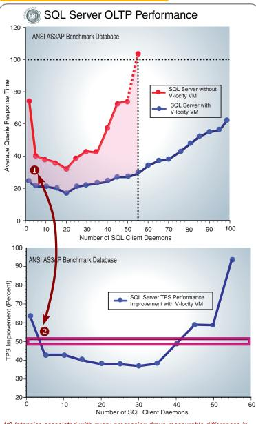
I/O latencies associated with query processing drove measurable differences in query response time • . Without V-locity VM, the average response time for OLTP queries was 128% longer. With faster response times, query TPS rates • averaged 50% higher, which enabled users to process more rows of data within a given time interval with V-locity VM.
