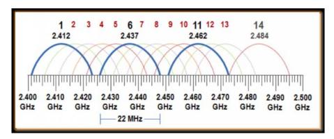
The diagram above depicts a spectrum analyser view of the frequency space occupied by these 14 channels. Within the 2.4 GHz band, only three channels have non-overlapping frequency space: channels 1, 6 and 11.
